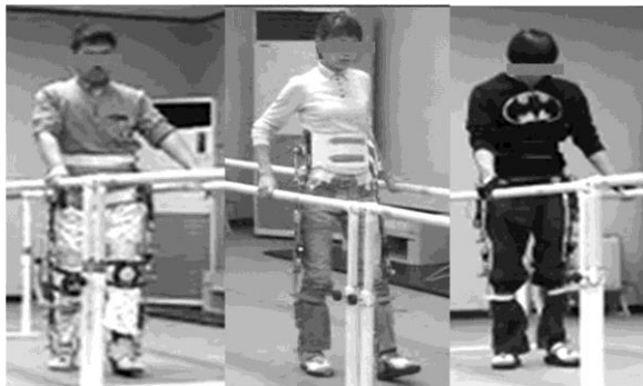
Fig. 4. Gait training of the powered orthosis
